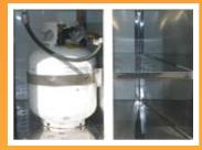
3. Propane tank/storage compartment consists of conventional lpg 5 gallon tank and regulator hose. Two adjacent storage compartments: 13" x 33" x 9"
